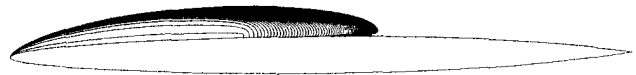
Fig. 5 Changes of the cavity shape with the iteration steps. (NACA 16-006, \alpha = 4 deg, \sigma = 0.87513 , l_{initial}/C = 0.37550 , converged l/C = 0.59279 .)
