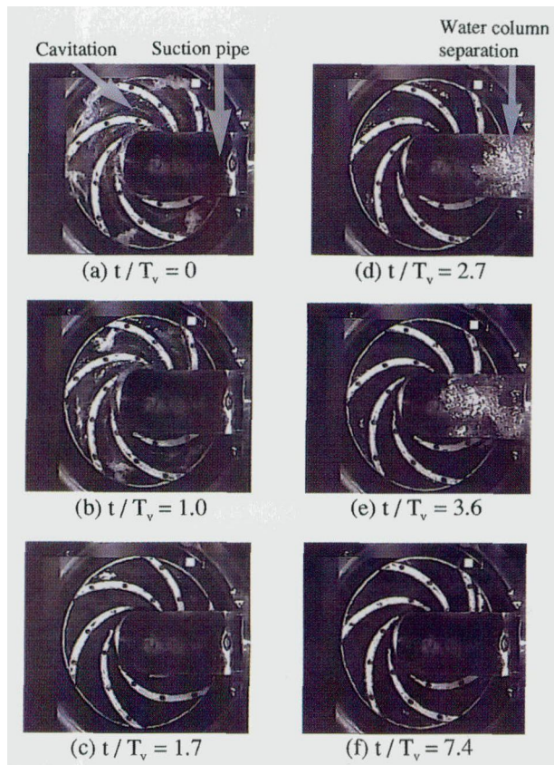
Fig. 11 Dynamic behavior of the cavitation at sudden closure of the discharge valve
